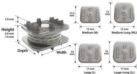
Figure 2: M6-C Artificial Cervical Disc Heights and Footprint Sizes
