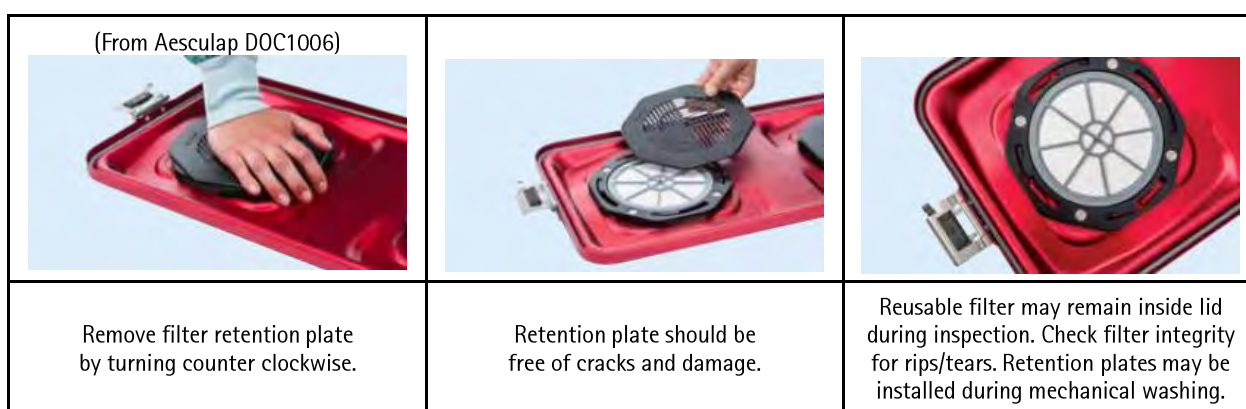
Figure 5: PrimeLine Pro Lid Inspection Process
