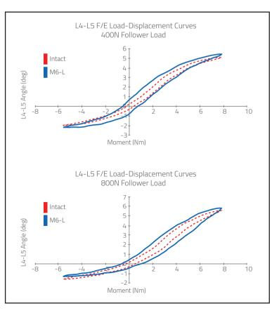
The "kinematic signatures" of the intact disc (red) and M6-L lumbar disc (blue) are nearly identical. The M6-L lumbar disc maintained total ROM, vs. Intact , at 400N [9.4°±2.2° vs. 8.8°±1.1°, p=0.56], and at 800N [9.5°±2.1° vs. 8.4°±1.2°, p=0.32], with excellent Quality of Motion.
