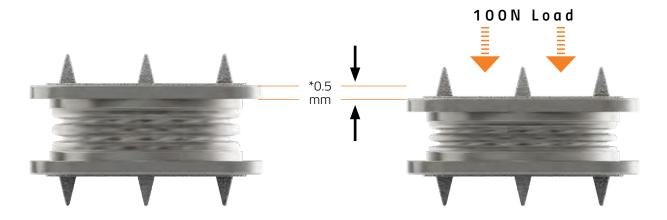
\*The M6-C artificial cervical disc compresses approximately 0.5mm under physiologic conditions (i.e. 100N Load, 37 deg C, Hydrated).
