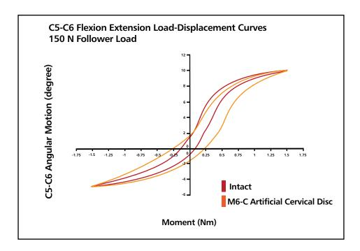
Biomechanical results showing the M6-C artificial cervical disc (orange) maintained total ROM (14.6) vs. the intact disc (14.4) with excellent Quality of Motion. The "kinematic signatures" of the intact disc (red) and the M6-C artificial cervical disc are nearly identical.
