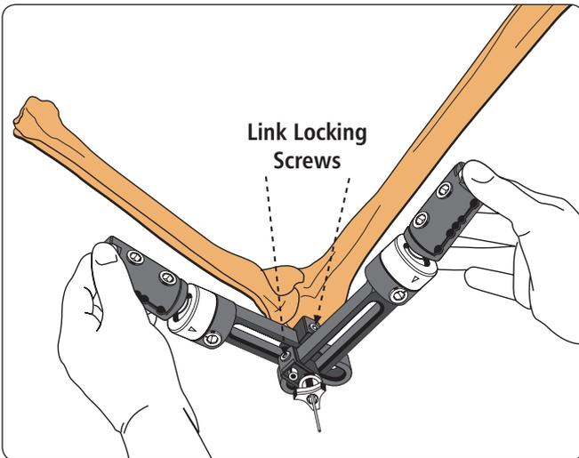
Slide the fixator over the 2mm Kirschner wire. Adjust the position of the links so that sufficient space is available for subsequent correction.
