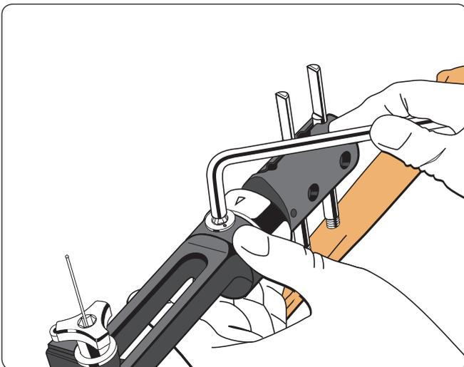
Finally, tighten the ball-joints with a 6mm Allen Wrench.
