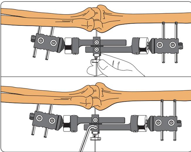
Lock the triangular knob and then each of the link locking screws.
