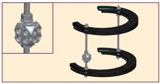
It can also be suspended on a threaded bar (lengths 80-120-160-200 mm, codes 80036-80037-80038-80039) between two rings.
