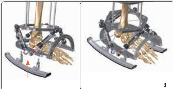
3. Place the TrueLok RockerRail with the FRONT marking anteriorly onto the Foot Plate by inserting its fixation rods into the appropriate holes
