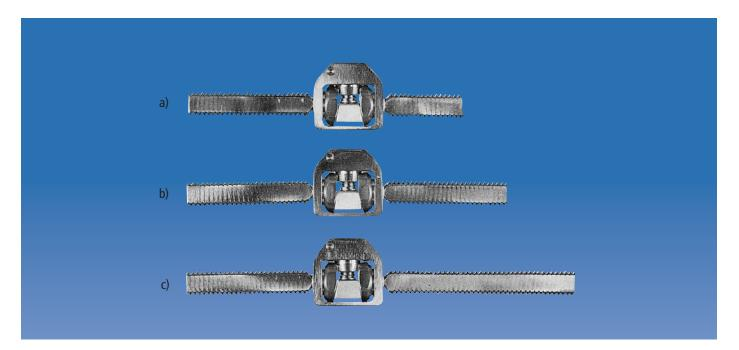
The central element of the Pennig Minifixator is a double ball-joint with a single screw locking mechanism embedded in a module 15.5x15mm square. The central element connects two threaded bars to constitute short (a) (bars 28.1mm and 18.1mm), standard (b) (both bars 28.1mm) and long (c) (bars 28.1mm and 43.1mm) Minifixators.
