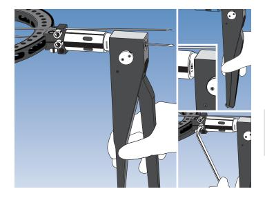
To tension wires, open handle of wire tensioning device to fullest extent.
