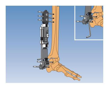
Attach the compression-distraction unit and distract the tibio-talar joint until 7-10 mm joint space is seen. Check that joint movement is adequate. Tighten the articulation locking nut with the ankle plantigrade.
