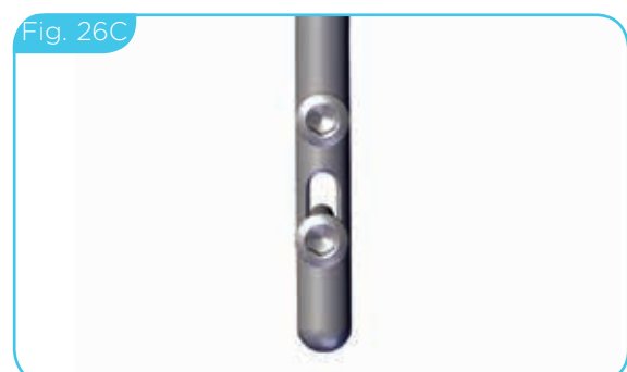
Static but potentially dynamic locking
